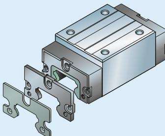
The seal kit consists of a metal scraper and an additional front seal. It is intended for applications involving exposure to coarse and fine dirt as well as liquids.
