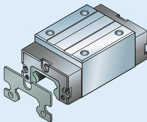
Scraper plates are spring-steel, non-contact components. They protect the front seal from, for example, coarse contaminants or hot metal chips.
