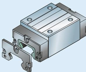
Additional front seals are contact seals that can be attached to the carriage end faces. They are single-lip seals consisting of special heavy-duty material and offer additional protection against liquids and smaller contaminants.
